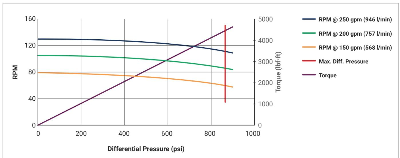
**Drilling Motor – Standard Series**
