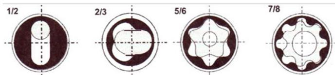
combination of the spiral shapes and lobes form sealed cavities between the two components. When drilling fluid is forced through the power section, the pressure drop across the cavities will cause the Rotor to turn.
