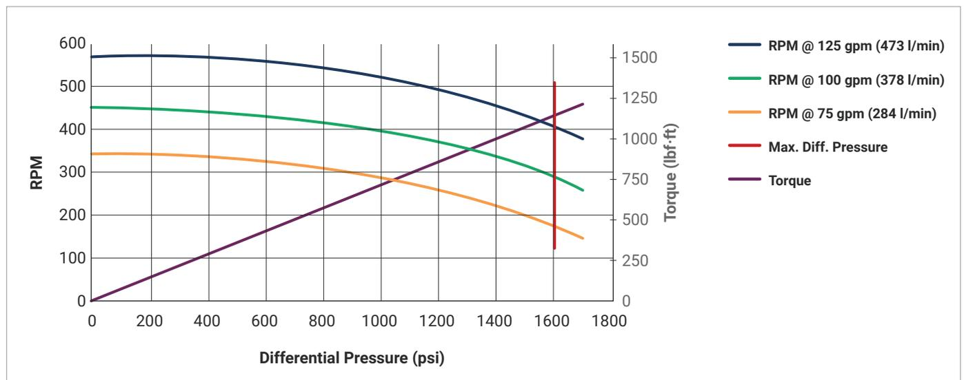
Drilling Motor – High Performance Series
