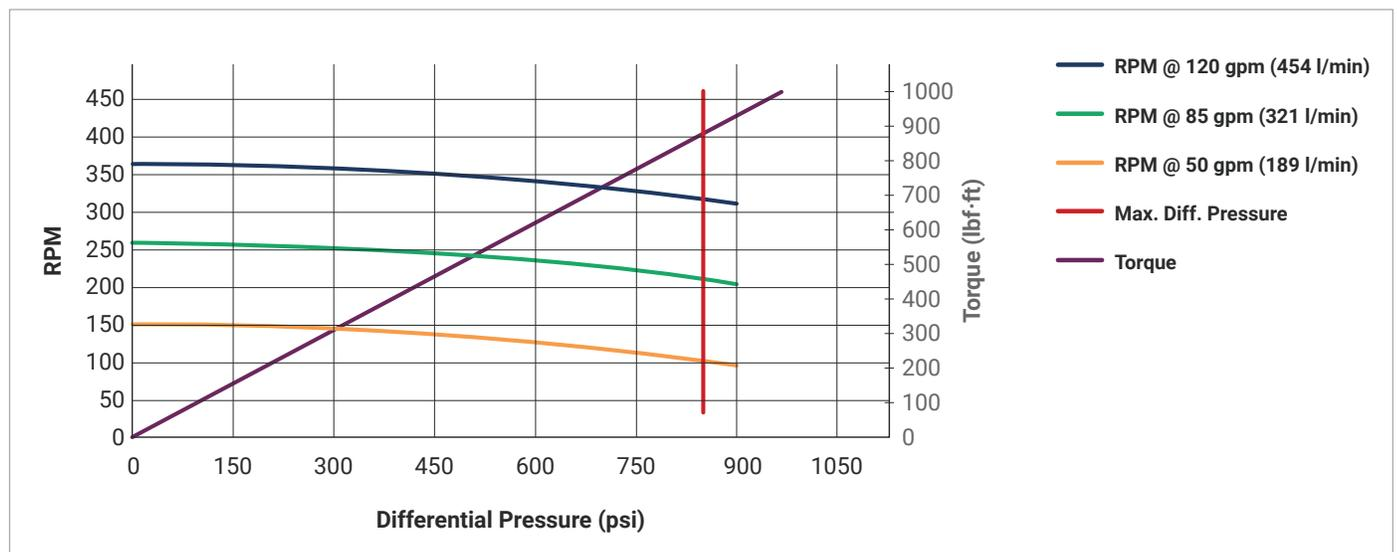
**Drilling Motor – High Performance Series**
