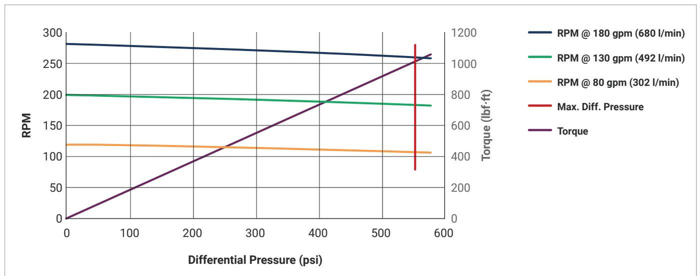
**Drilling Motor – Standard Series**
