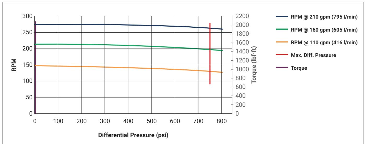
Drilling Motor – Standard Series
