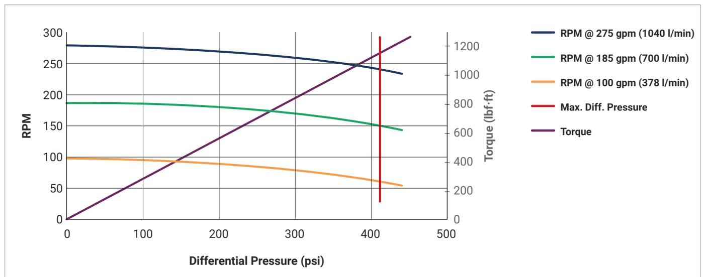
**Drilling Motor – Standard Series**
