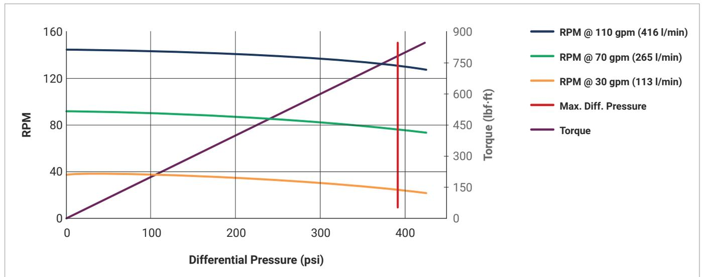
Drilling Motor – High Performance Series
