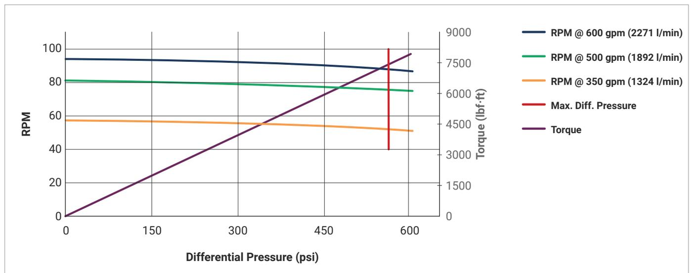
Drilling Motor – Standard Series
