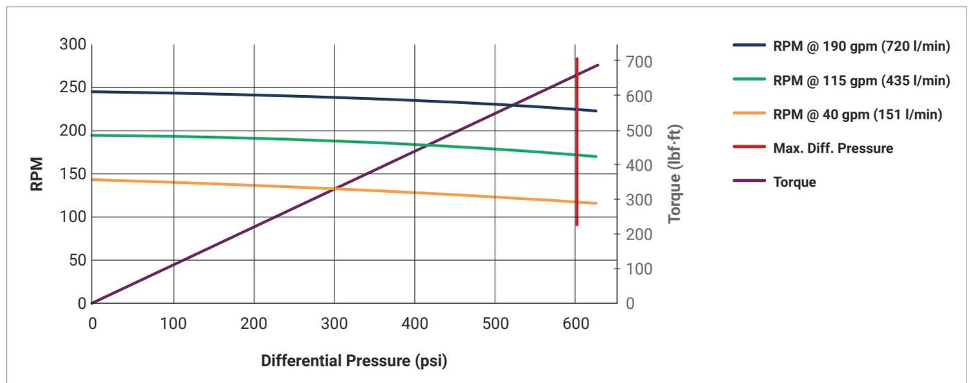
**Drilling Motor – Standard Series**
